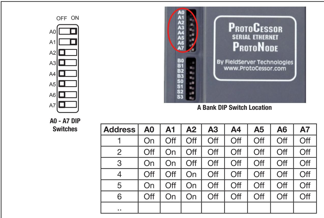
**Figure 5: Switch Configuration for MAC Address**
