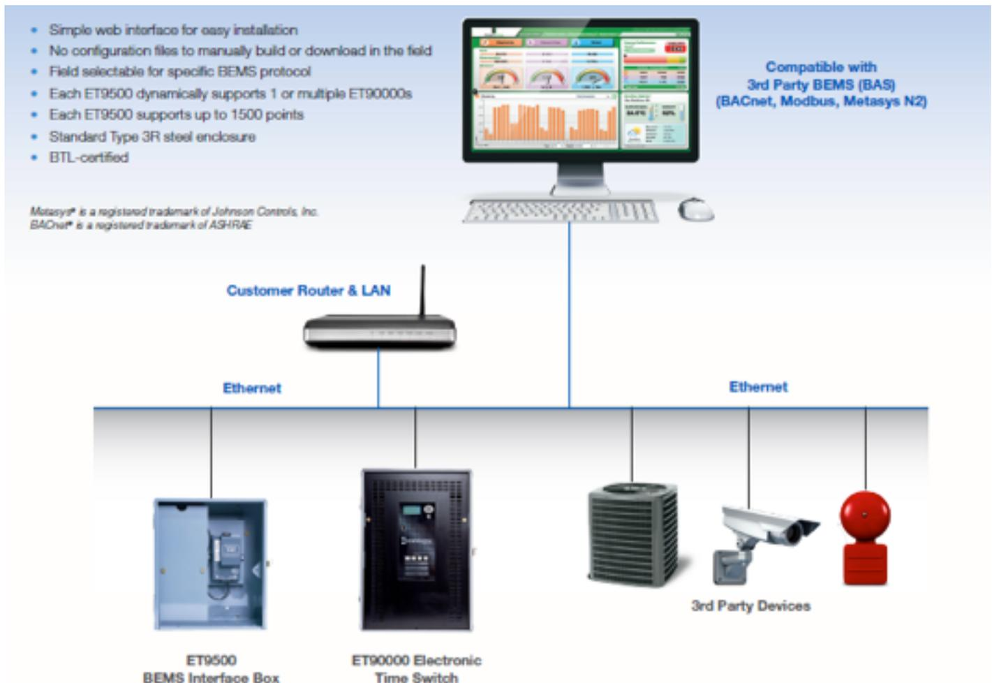
Figure 1: System Configuration
