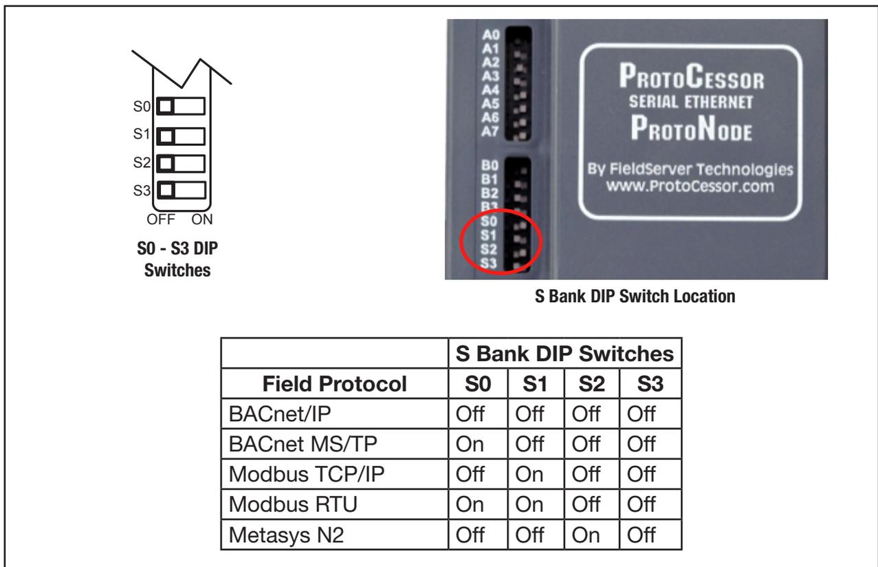
**Figure 3: Switch Configuration for Field Protocol**
