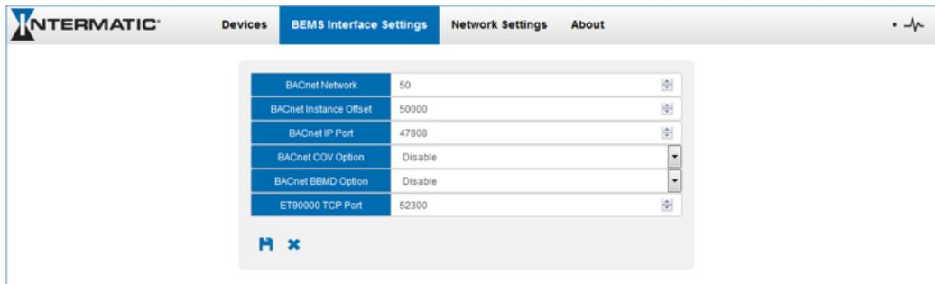
Figure 20: Web Configurator showing setting the network number for BACnet IP
