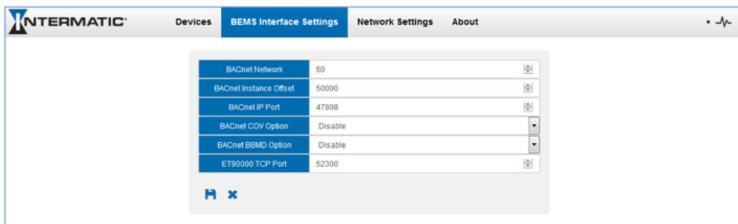
Figure 21: Setting up the ET9500 for BBMD on the BACnet IP Network
