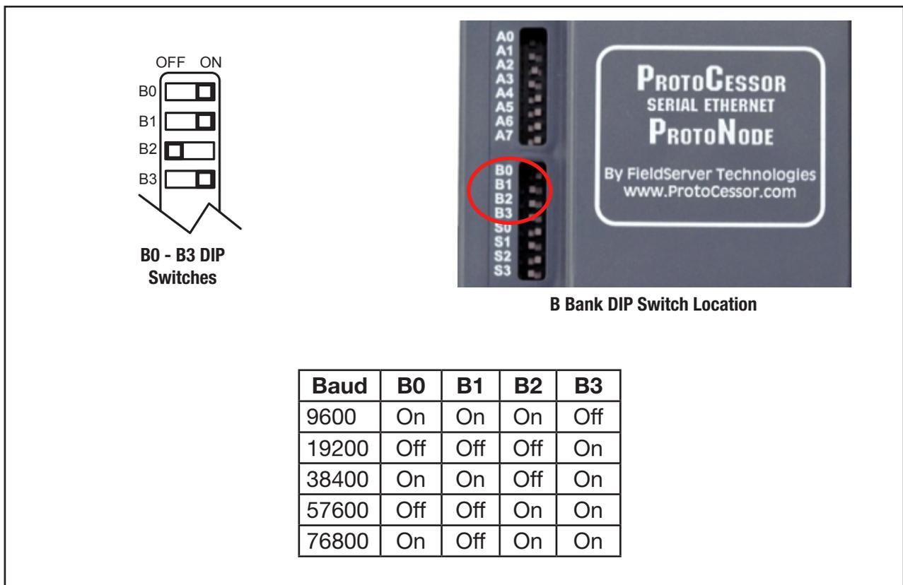
**Figure 4: Switch Configuration for Baud Rate**
